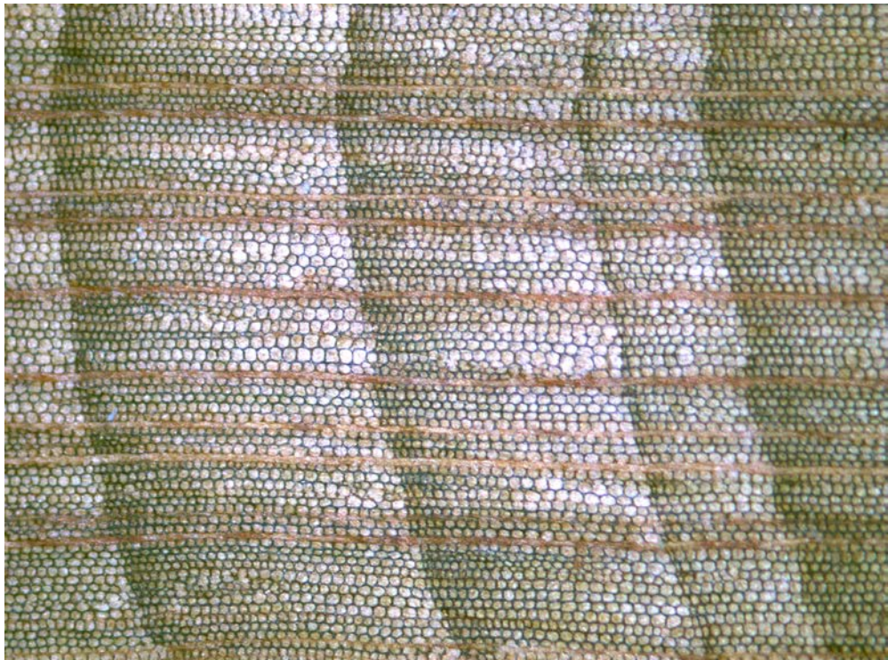
Three kauri tree rings. The line of dark (thick walled) cells indicate the end of the growing season. Growth is from right to left.
